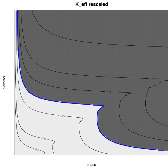
Figure 1: k_{\text{effective}} evaluated on a regular grid on [0, 1]^2 . In blue the contour line k_{\text{effective}} = 1 , the true safe region is the light gray area.
